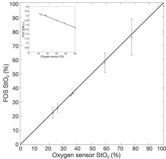
**Figure 3** Capillary filled with human hemoglobin, different oxygen saturation values were obtained and measured with a bench-top oximeter. FOS, Flow Oximetry System; StO<sub>2</sub>, oxygen saturation.
